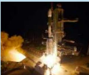
The GSLV-F10 is a three stage/engine rocket. The core of the first stage is fired with solid fuel and the four strap-on motors by liquid fuel. The second is the liquid fuel and the third is the cryogenic engine.
